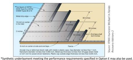
ynthetic underlayment meeting the performance requirements specified in Option E may also be use Sealed Roof Deck Option <u>D</u> or <u>E</u> [NOTE: E is NOT an Option for Wood Shake/Shingle]
